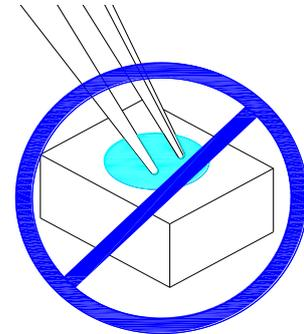
2.The outer diameter of the SMD pickup nozzle should not exceed the size of the LED to prevent air leaks. The inner diameter of the nozzle should be as large as possible. A pliable material is suggested for the nozzle tip to avoid scratching or damaging the LED surface during pickup. The dimensions of the component must be accurately programmed in the pick-and-place machine to insure precise pickup and avoid damage during production.
